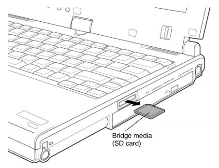
Figure 4-3 Removing the Bridge media
